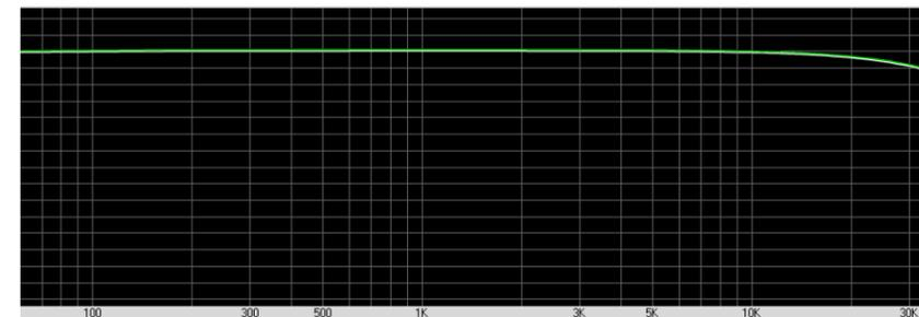
Graph 2: Frequency Response using 24-bit/96kHz data.
