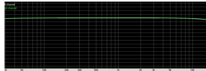
Graph 1: Frequency Response using 16-bit/44.1kHz data.
