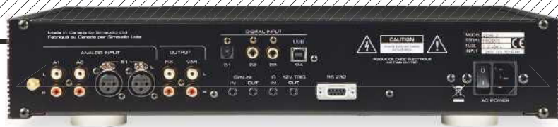
ABOVE: At the rear are balanced and unbalanced analogue inputs and, if the unit has the optional built-in DAC, a set of digital inputs including Toslink optical, two coaxial (S/PDIF) connections and USB. The RS-232 port allows for firmware updates
