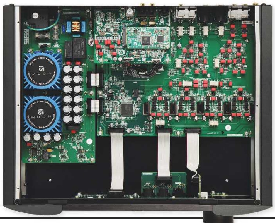
RIGHT: In addition to Simaudio's dual-mono PSU and 'M-LoVo' four-stage voltage regulation (left-most PCB) our sample has the ES9018-based DSD256/384kHz DAC board fitted
