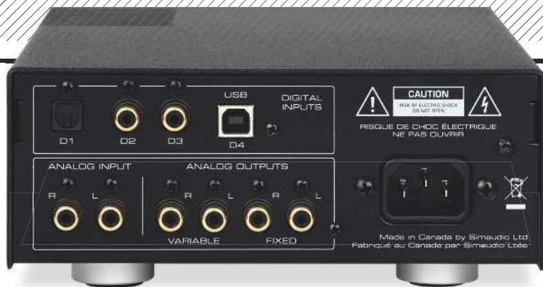
ABOVE: A comprehensive suite of digital inputs is offered (including 384kHz/32-bit USB and 192kHz/24-bit S/PDIF on coax and optical) plus one set of analogue inputs on RCA. The analogue outputs are offered at a fixed 4V or variable, both on RCAs
