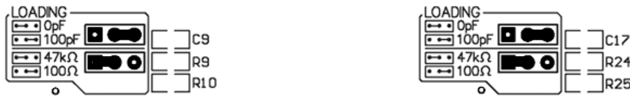
Figure 2: Left and right channel jumper banks for moving magnet (default) loading adjustments
