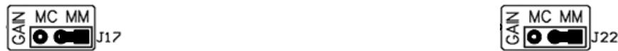
Figure 3: Left and right channel jumper banks for moving magnet (default) gain adjustment
