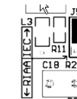
Figure 7: IEC Equalization curve jumper setting
