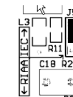
Figure 7: IEC Equalization curve jumper setting
