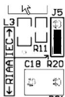
Figure 6: RIAA Equalization curve jumper setting
